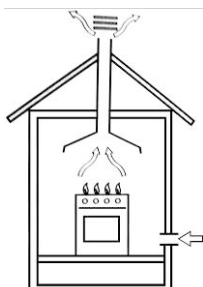
In a chimney stack or branched flue.
